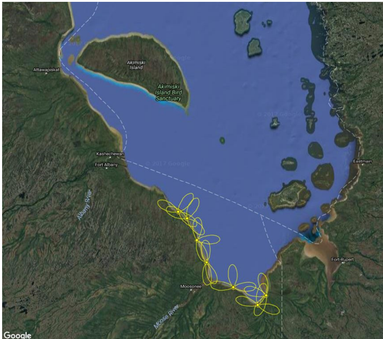
Figure 2. Locations of the project's seven Motus towers, showing direction and relative coverage of antennas. Active 17 May to 1 December 2016.
